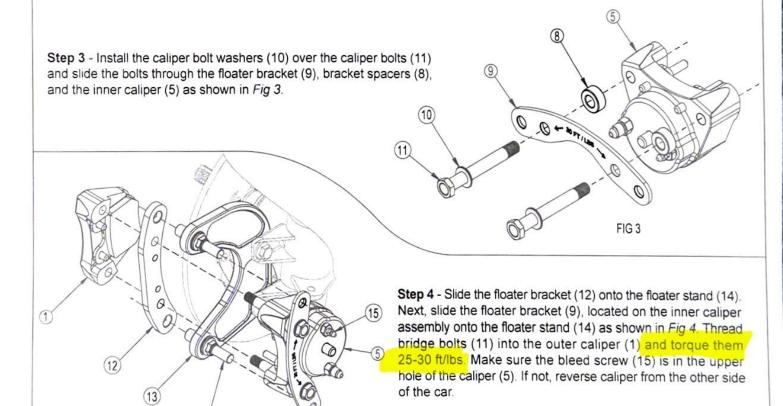
NOTE: When the pin in the center of the caliper is almost flush with the caliper housing, its time to change the pads. Do not operate car beyond that point, or fluid loss and brake failure will result. When worn, the inner caliper pad can be resurfaced to become a new outer pad
